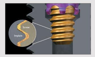
Fig. 6. Gold-Tite<sup>®</sup> Abutment Screw (BIOMET *3i*). The gold coating acts as a dry lubricant to reduce friction between the screw and the implant threads.
